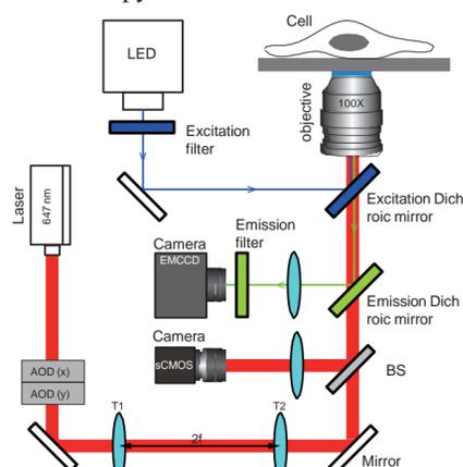
AOD: acousto-optic deflector, BS: beam splitters, T1-2, telecentric lens (f = 500 mm), Excitation/emission wavelength (482/520 nm)
