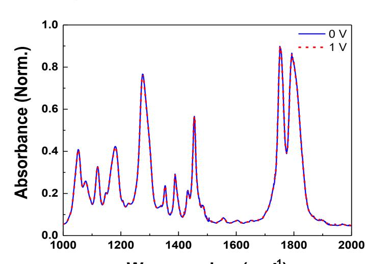
Wavenumber (cm<sup>-1</sup>) The FT-IR spectrum of DMC/PC(1:1 v%) with electric potential.
