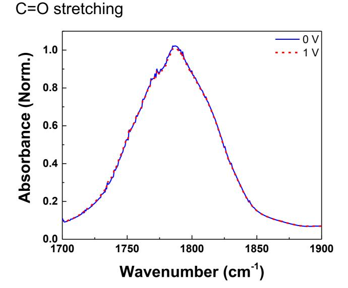
The FT-IR spectrum of 1 M LiPF<sub>6</sub> in PC with electric potential.
