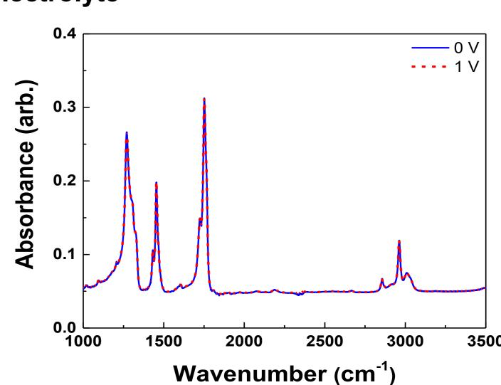
The FT-IR spectrum of 1 M LiPF<sub>6</sub> in DMC with electric potential.
