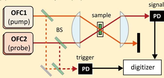
The schematic diagram of DFC linear spectroscopy (a) and DFC-TA.  $f_r = 80$  MHz,  $80$  MHz +  $\Delta f_r$  for OFC1 and OFC2, respectively. Every signal pass through a 48 MHz low-pass filter LO: local oscillator, PD: photodetector, BS: beam splitter.
