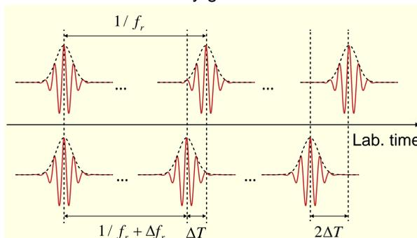
By detuning the repetition rates of two independent frequency combs, a time-delay is generated with an increment  $\Delta T$
