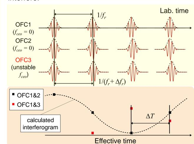
When  $f_{ceo} = 0$ , the optical interference in DFC system arises at a down-converted frequency  $f_{RF}$
