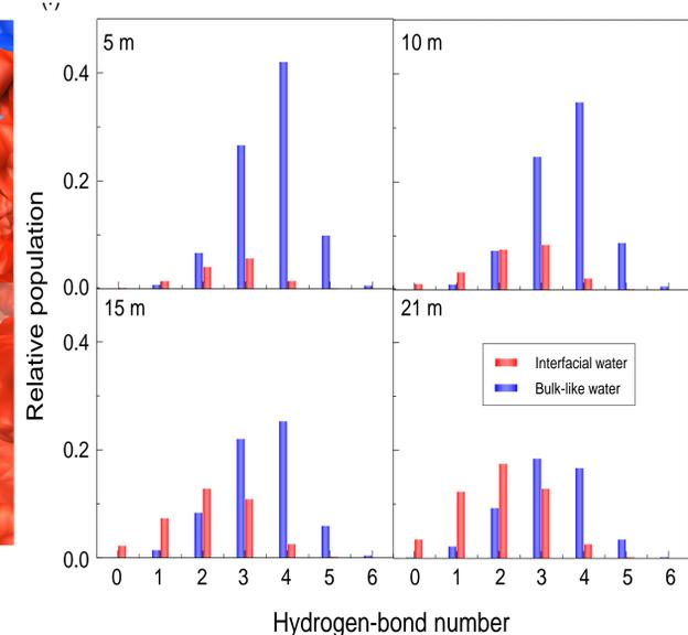
Histogram of H-bond number per water molecule and relative population of bulk-like water and interfacial water molecules
