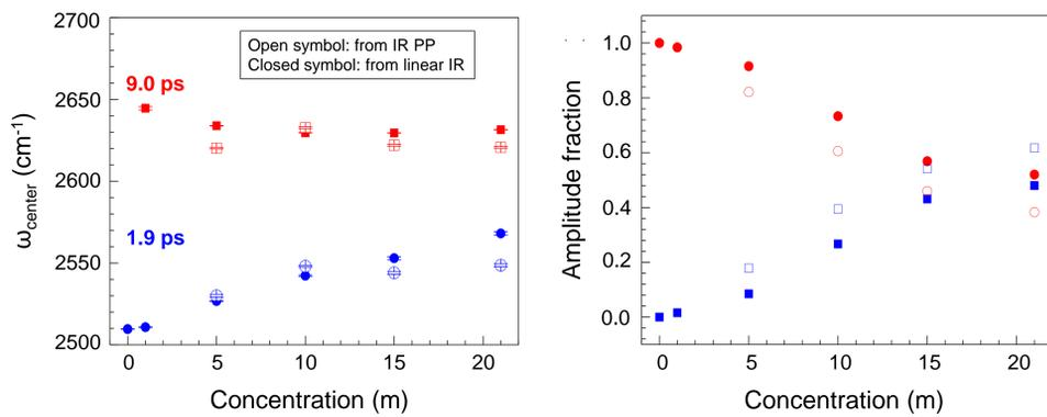
(Left) Center peak frequency and (Right) amplitude fraction of water species Both information was obtained by Gaussian fit on FT-IR and isotropic signal at several concentration (5-21 m).
