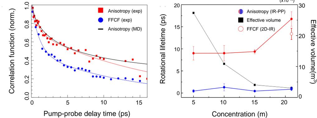
(Left) Rotational (anisotropy, PSPP) and spectral diffusion (FFCF, 2D-IR) correlation function and (Right) rotational decaying constant and corresponding effective volume of water in ionic system.
