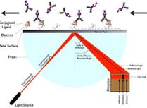
SPPs are propagating waves along a metal-dielectric interface. Because of high field enhancement, SPPs are used on biosensing application.
