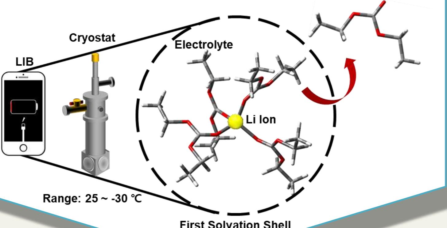
Lithium-ion battery has received much attention due to the high power density and good rechargeability. However, the application of the battery is limited at a low temperature, in that it shows poor performance in the unexpected cold due to the increasing impedance of charge transfer. To break through the current state, we are trying to get information about the change of the solvation structure of LIB at low temperature with a cryostat.
