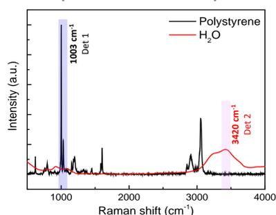
→ The resonant CARS signals from each target molecules in the sample (polystyrene) and the surrounding medium (water) divided by the dichroic mirror are separately detected by two PMTs in simultaneously.
