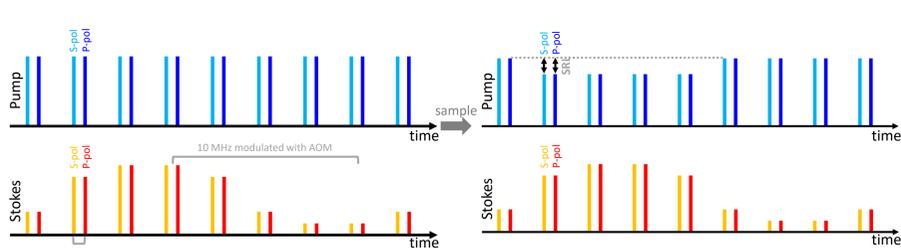
S-pol and p-pol pump pulses are targeted at different Raman shift. SRL signals are collected with separated photodiodes then transferred to different signal-in channel of lock in amplifier.
