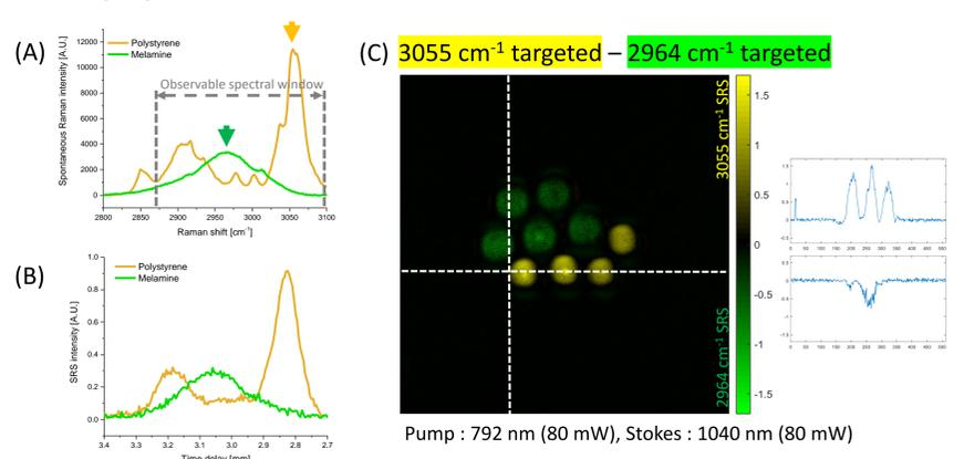
(A) Measured spontaneous Raman spectra of polystyrene and melamine. (B) Corresponding SRS spectra of polystyrene and melamine. (C) Real-time two-color SRS image of  $9 \mu\text{m}$  polystyrene beads and  $10 \mu\text{m}$  melamine beads mixture. Calculated signal to noise ratio is 51.28 and 28.45 each.
