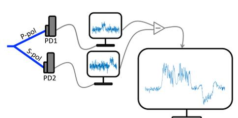
Since both two pairs of pump and Stokes experience the same environmental condition at the sample position, a simple balancing procedure between SRS processes of two different vibrational modes can decrease background noise level without signal loss. Since two SRL signals are subtracted, they give opposite signs of signal.
