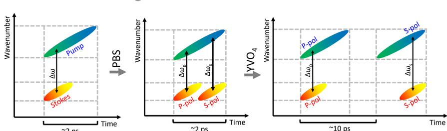
Delay stage 2 containing polarizing beam splitter enables orthogonal polarized pulses to target two different Raman shifts in spectral window of  $130 \text{ cm}^{-1}$ . Birefringent material YVO<sub>4</sub> generates additional time delay about 10 ps. Since two orthogonal pump and Stokes pulses are timely distant, no optical coherence can occur.
