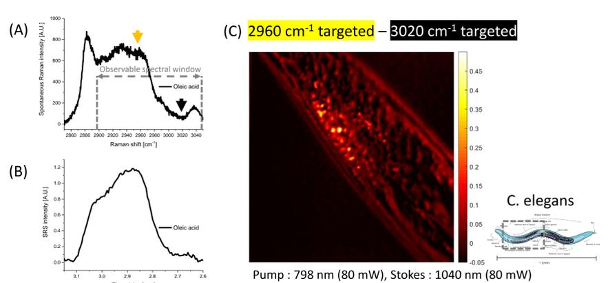
(A) Measured spontaneous Raman spectra of oleic acid. (B) Corresponding SRS spectra of oleic acid. (C) Real-time two-color SRS image of C-elegans at  $2960 \text{ cm}^{-1}$  as on resonance and  $3020 \text{ cm}^{-1}$  as off resonance.
